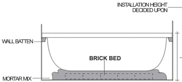
The battens must be securely mounted ( we suggest rawl bolts) Mix up sand into a dry mix at a ratio of 5:1. This will be used to form a secure bed, which will support the bath. Approximately two wheel barrow loads will be required.
